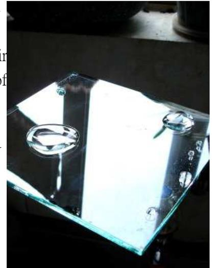
The surface of EJ Glass has high hydrophobic property which is similar to lotus leaves. The rain drops do not stick on the surface, but form water drop shape because of its surface tension. The rain drops slip down and carry the dust away in the mean time. This gives the glass with easy cleaning advantage and the dust will not accumulate on the surface. Comparing with normal glass, it results the obvious difference in the long term.
